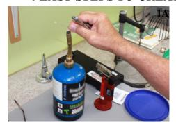
Warm clasp by lightly waving it over flame. (WARNING: DO NOT OVER HEAT THE CLASP)
