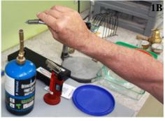
Lightly pass 3 prong plier over flame. (WARNING: OVER HEATING PLIER WILL CAUSE INDENTATION IN CLASP)
